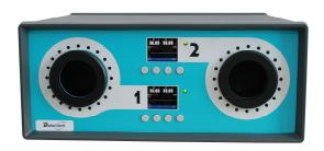
The BL672D is a benchtop blackbody calibration source utilizing a digital indicating temperature ambient 30°C to 50°C (86F to 122F). Two 60mm diameter end closed tube is heated or cooled with an internal solid state thermoelectric heat pump. It has a built-in digital temperature controller to provide accurate, stable temperature as well as to provide readout.
